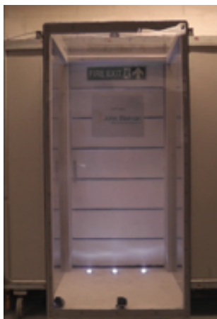
Smoke seals fitted head and jambs
